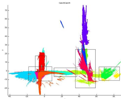
**Figure 8:** Sample tracks for all cameras; each color denotes all tracks observed by a given camera; boxes denote regions of high overlap between cameras.
